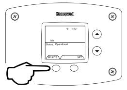
Step 2: Press "Set" button to change temperature format. "°F/°C" symbol will flash in the water heater display.
